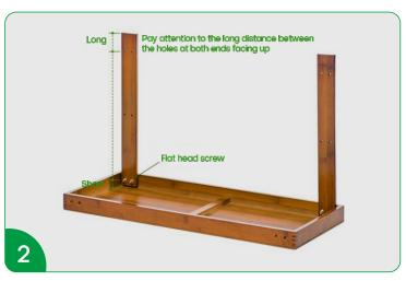
Take out 2 flat head screws of the tripod and install as shown in the figure, with the long holes facing upwards.
